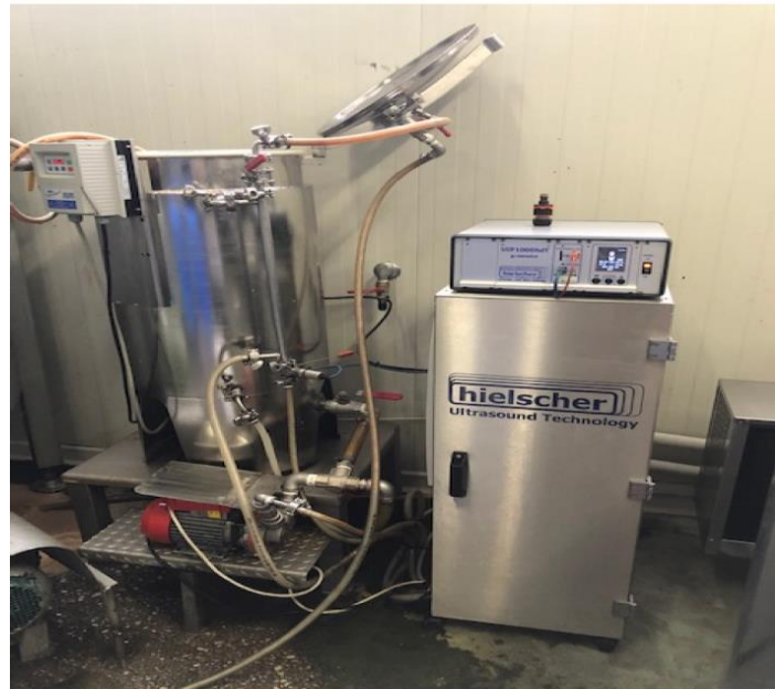
Figure 2. The continuous ultrasonic homogenization device (type UIP1000hdT (1000W, 20kHz) supplied by German company Hielscher Ultrasound Technology.
