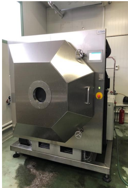
Figure 1. The morphology of the industrial type lyophilizer of POLYHEALTH S.A. which was used in the experimental project.
